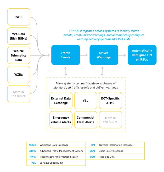
Figure 1: Key components of the CIRRUS platform.
